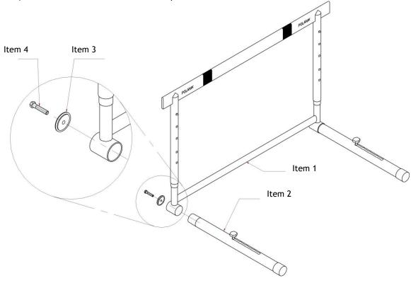
The main goal of the hurdle collapsible construction is to assure easy and cheap transport. Note that once you screw the feet down, the hurdle is practically non-dismountable. Therefore we do not recommend unscrewing the hurdle feet during idle periods. Removing the feet without proper tools can cause serious hurdle damages which Polanik shall not be liable for.
