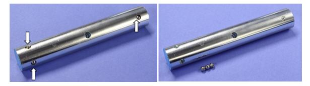
h) the counterweight, the ball sockets and the inside of the foot tube should be cleaned from dirt and old grease, i) grease the inside of the ball sockets and install the balls,
