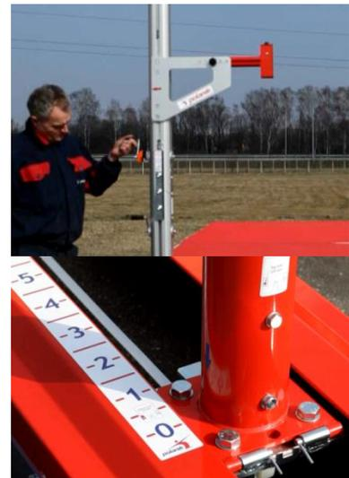
3. While 2 people are securing the post as high above the hinge as possible, loosen the screws of the blocking bar, slide down the blocking bar to unlock the hinge.
