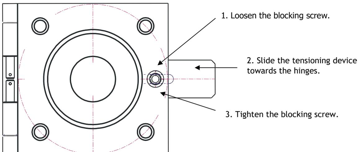
Now tighten the nuts (you have screwed temporarily in base side plates) with wrench. Correctly tensed cog belt should deflect no more than 2 cm approx. when pressed with index finger. Cog belt tensioning should be done scrupulously. If cog belt is too loose, it may slip on toothed wheels in post sliding mechanism. On the other hand, when cog belt is too tense, it may cause too high resistance and load of sliding mechanism.
