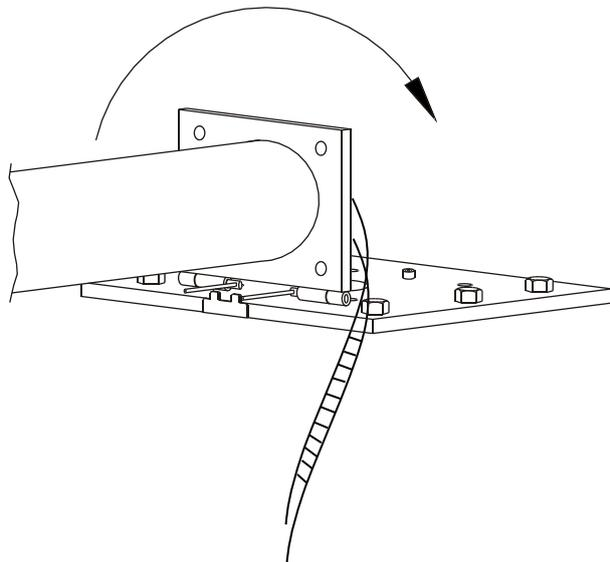
While holding the cog belt ends under the trolley plate, lift post to the upright position.
