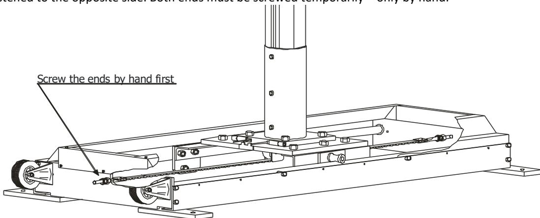
Make preliminary tensioning with tensioning device (see image below). Base trolley – top view
