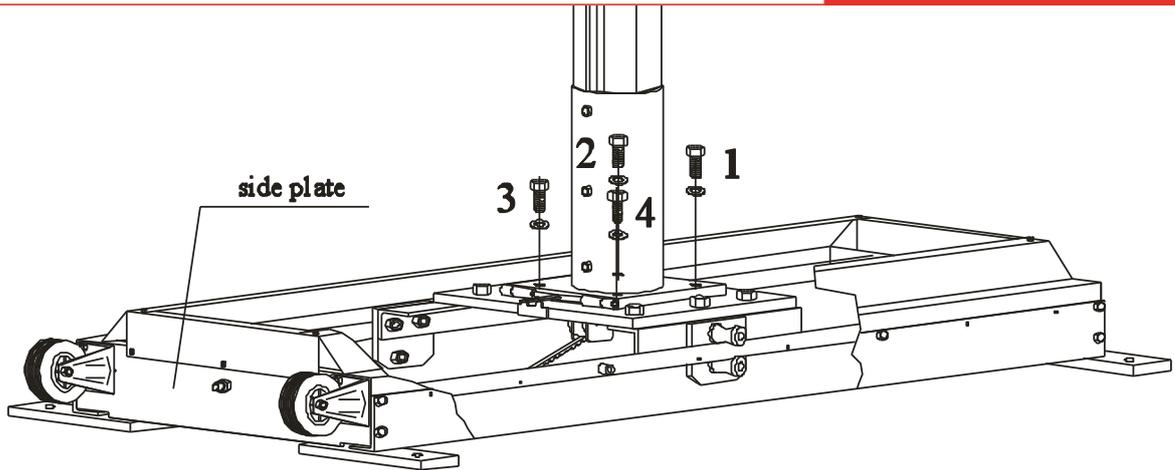
Screw down the screws which are opposite the trolley hinge first. Next remove safety. **Safety bar should be kept for further use – it makes the disassembly process and transport of STT15-65F easy and safe.** Now install the cog belt ends. One end should be screwed to the base side plate where safety bar has been mounted and the other one ought to be fastened to the opposite side. Both ends must be screwed temporarily – only by hand.
