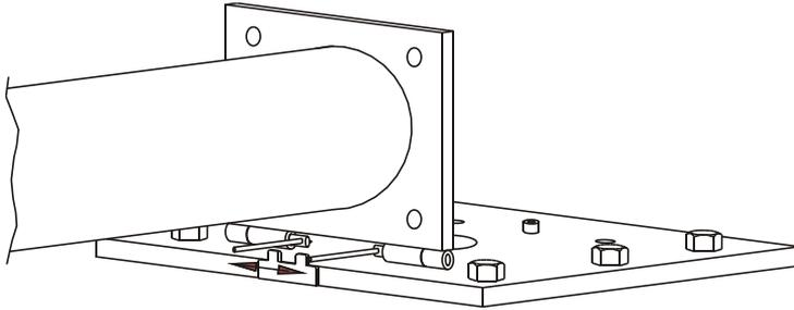
Release hinge pin levers, which spring back automatically to their working positions and connect post foot with base trolley. That pivotal joint is used to put posts in the upright position.
