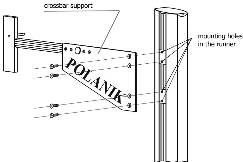
Next screw down crossbar supports to the posts while they are resting on the ground. Use 4 countersunk screws for each support. The screws are temporarily mounted in the runners of the posts.
