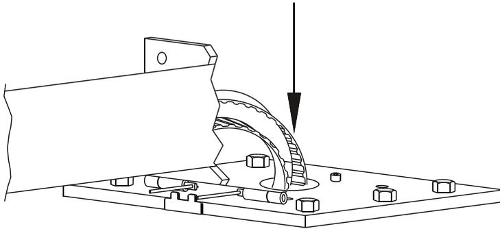
Pull out the cog belt ends from post profile and thread them through the hole in base trolley
