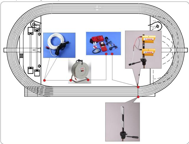
At the start line the starter fires the starting revolver RS-START9, which is connected with the chronometer CHR through the 150 m cable PNB-150. At the finish line the two sports photocells FP are screwed to the cascade holder UFP-2 and mounted on the tripod ST. they are connected to the chronometer CHR. The photocells are pointed to the double reflector LFP-2 mounted on the tripod ST.
