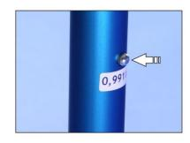
c) next the hurdle toppling force should be adjusted accordingly, so pull and hold the knob in the hurdle foot,
