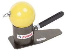
Press the lever all the way down - the steel sleeve (diameter 12 mm) lifts the hammer head (shot put) from the edge. If the hammer head (shot put) stays on the sleeve, it complies with the IAAF rules.
