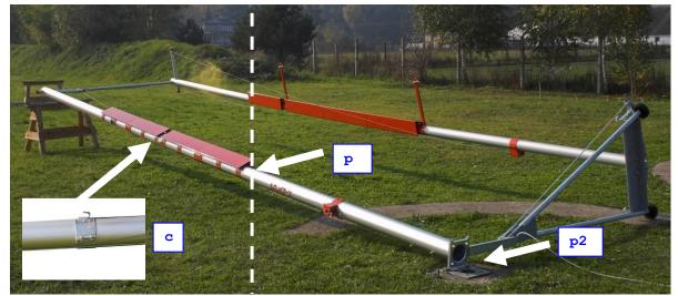
After erecting the gate and fixing its wings by following the instruction, the shields tip should aim to the center of the circle. Properly installed shields are shown below.
