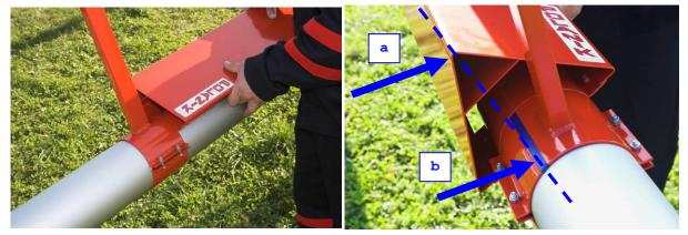
After the shield frame being fixed properly, screw the clamping rings (2) using screws (3) and washers (4).
