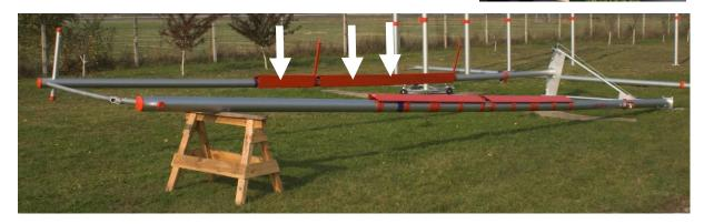
Fix the extreme pillar shields OS296 on the pillar with diameter 150 mm. The shield tips during fixing on the gate prepared for lifting should aim upward while the shields side coverings (p1) have to be put in parallel with the extreme pillar base edge (p1) – looking from the inside. Place the shields over and below the steel wire catch (c), which should be installed in compliance with the instruction manual of the cage gate lift CGL-3.
