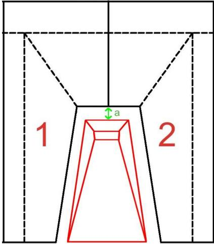
place the pole vault box surrounding pads (01 and 02 see the drawing on page 03) around the pole vault box, so as the distance between the rear edge of the box and the landing area pads (a) is 15 cm, make sure that all the Velcro® pads adjoin properly, next attach front panels 03 and 04,
